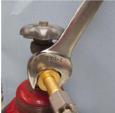
Connection of the Tank Reducing Union. Make sure to install the White Teflon gasket
